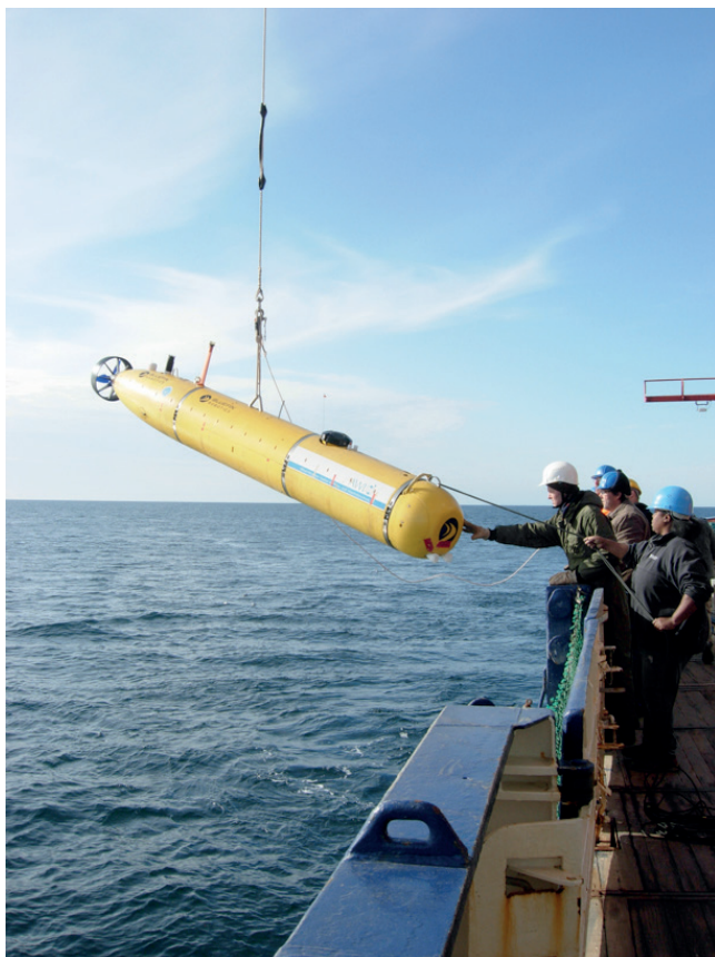
Fig. 3.1.1: Deployment of the Autonomous Underwater Vehicle
