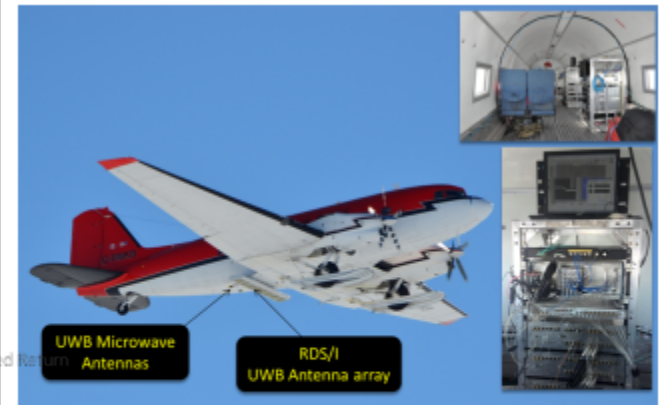
Figure 1. Photograph of the BT-67 (BASLER) platform outfitted with the radar antennas. The inset shows a photograph of the inside of the cabin equipped with the instrument package (top) and a photograph of the radar electronics (bottom)
