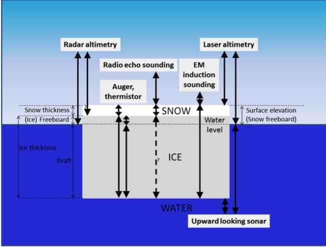
**Figure 4.1:** Cross section of an ice floe in isostatic equilibrium, illustrating variables comprising ice thickness. Observables retrieved by various ice thickness measurement methods are indicated by thick arrows.
