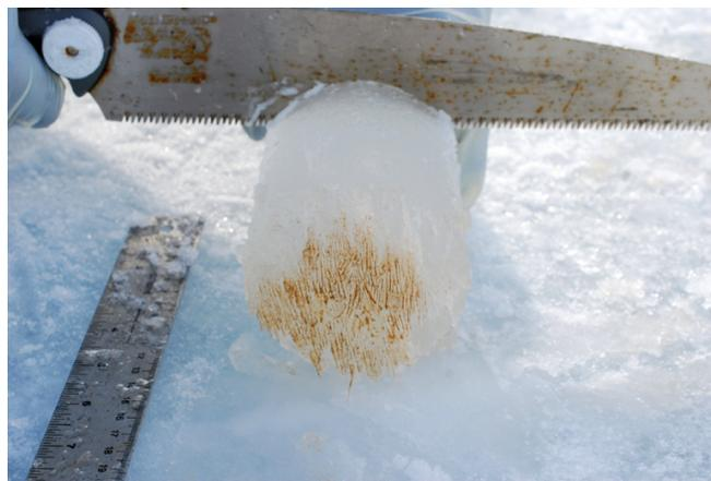
**Figure 8.1:** Sectioning of an ice core with a stainless steel hand saw on site. Note the discoloration due to microalgae in the bottom-most layer, with algal cells concentrated in brine layers between lamellar ice crystals.
