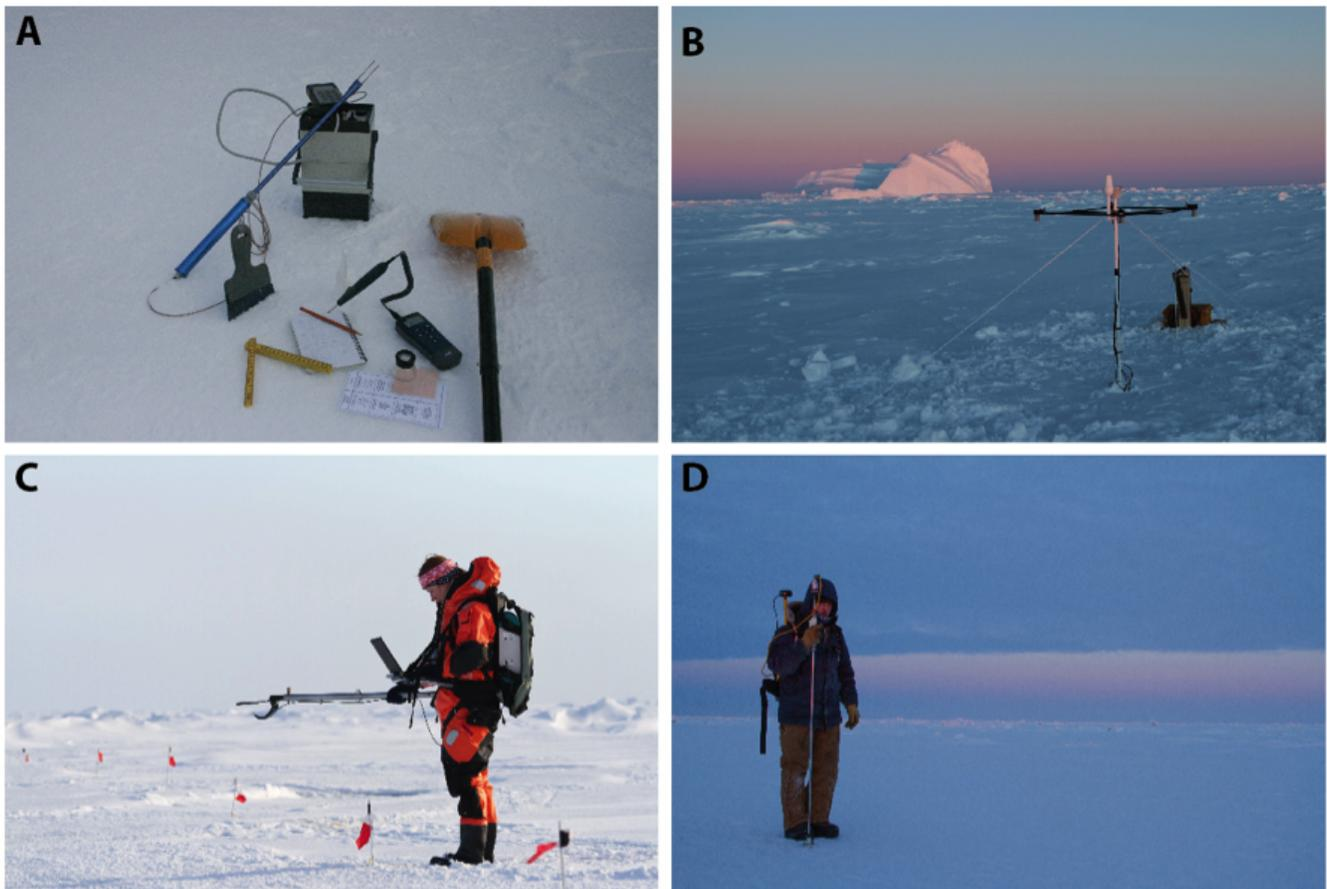
**Figure 3.1:** (a) tools for snow measurements in a snow pit (thermometer, density sampler, mm-grid), (b) snow depth buoy on Antarctic sea ice, (c) spectral albedo measurements with an ASD Field spec on Arctic sea ice during summer, (d) Magna Probe snow depth transect on land-fast sea ice in Barrow, Alaska.
