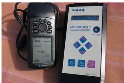
Fig. 3: Microtops handheld multichannel sun photometer (right) and attached GPS receiver (left). (Photo: Bernhard Pospichal)
