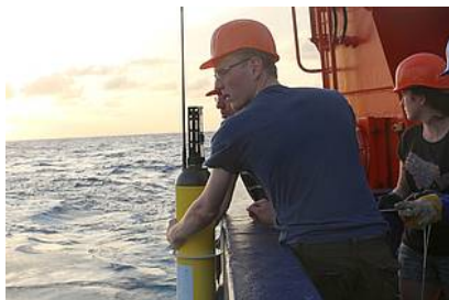
Fig. 2: Deployment of an ARGO-Float (Photo: Tobias Küchler, TROPOS)
