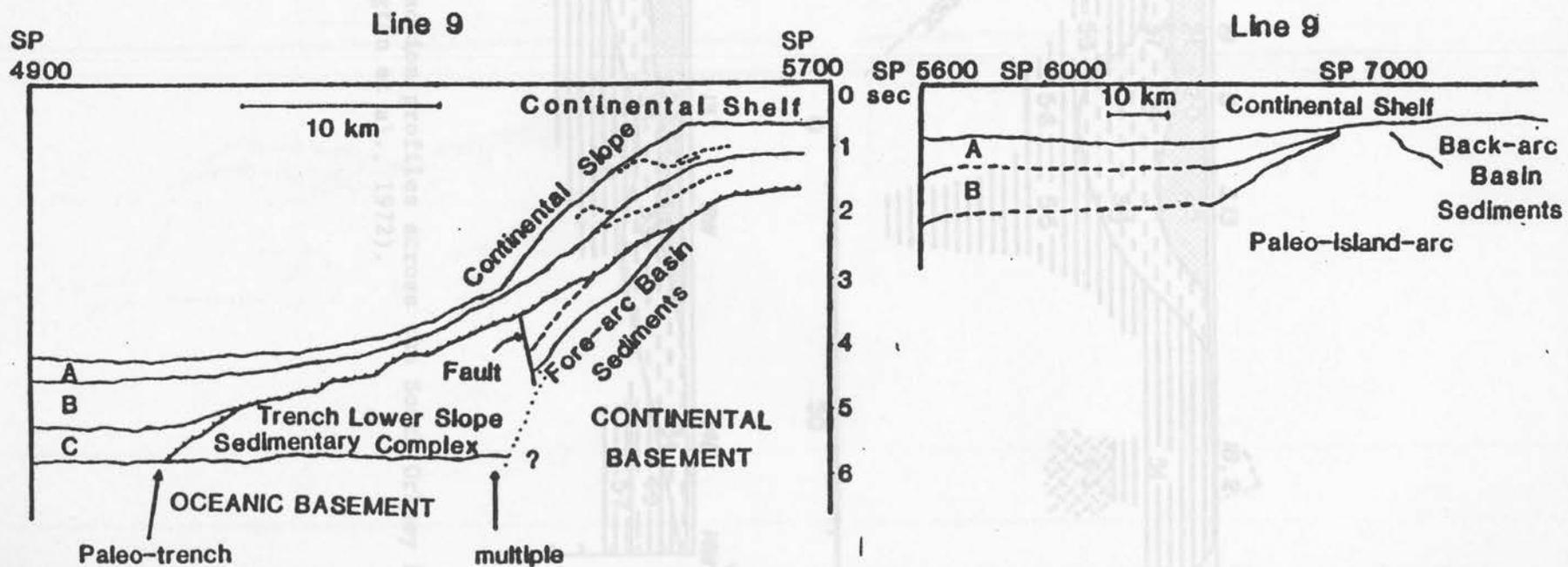
Figure 20. Interpreted seismic reflection profile across the Bellingshausen continental margin (from Kimura, 1982)
