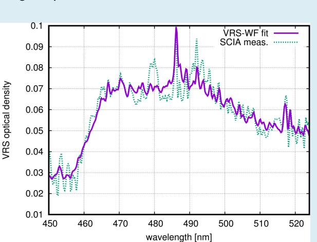
Example of a VRS weighting function fit at a oligotrophic site over the South Pacific on the 23 October 2008. The solid line is the scaled VRS reference spectrum and the dashed line is the measuremend subtracted all considered parameters except VRS
