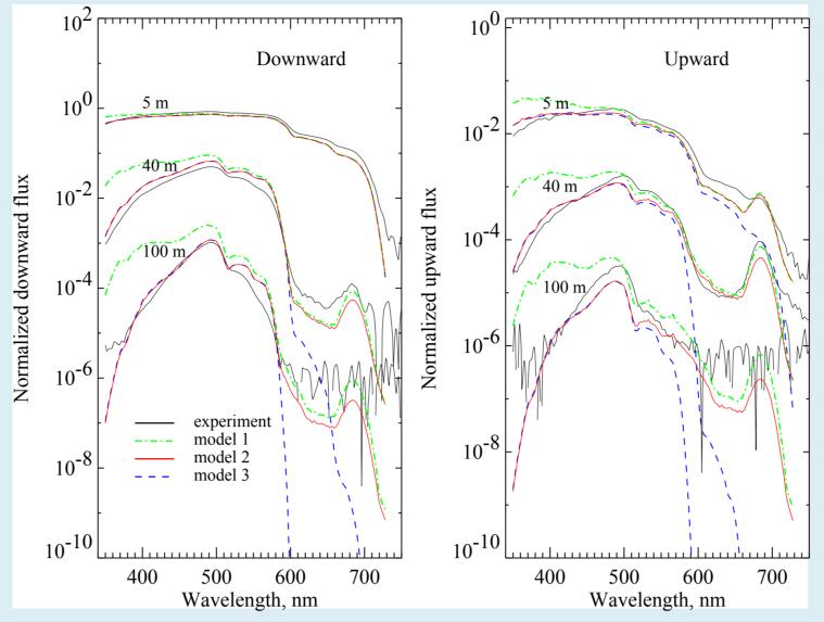
Comparison of measured and modeled spectral distribution of the down- and upwelling underwater normalized fluxes at three selected depths: "model 1" -simulations including VRS, CDOM and chl-a fluorescence. "model 2" - simulations as in "model 1" with two and a half times larger concentration of fulvic and humic acid; "model3" simulations as in "model 2" but excluding all inelastic processes.
