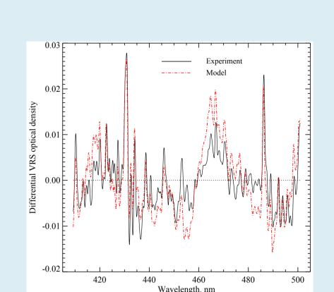
Experimental and modeled differential VRS spectra. Solid black line: Retrieved from MAX-DOAS measurements [51]. Dash-dotted red line: Calculated using SCIATRAN with the geometrical settings according to the ground-based measurements performed during the TransBrom campaign.
