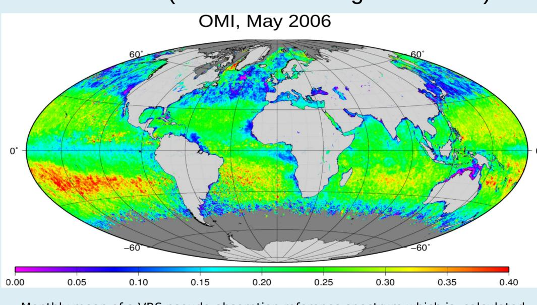
Monthly mean of a VRS pseudo-absorption reference spectrum which is calculated by SCIATRAN and fitted in a wavelength window of 446-497nm. Considered in the fit are also absorption of atmospheric trace gases, atmospheric Ring effect and a weighting-function for other oceanic parameters
