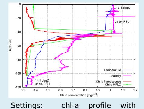
maximum of 1.025 mg/m<sup>3</sup> at 40m depth, measured on vessel campaign 15 May 2008 at 40.81N, 10.68W. Absorption is calculatet by CASE 1 water model [Morel&Maritorena, 2001]. SCIATRAN demonstrates ability to reproduce realistic light
