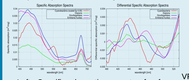
Left: Specific absorption spectra for four different PFTs from in-situ measurements. Right: Differential absorption spectra for four different PFTs.
