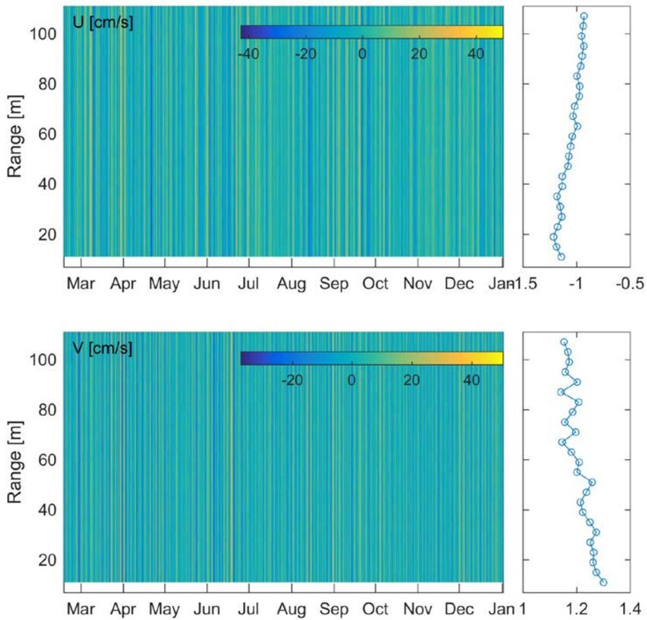
Figure 9. RDI ADCP SN 8645 (Longranger). Vertical range - time maps of east and north velocities and their time average profiles
