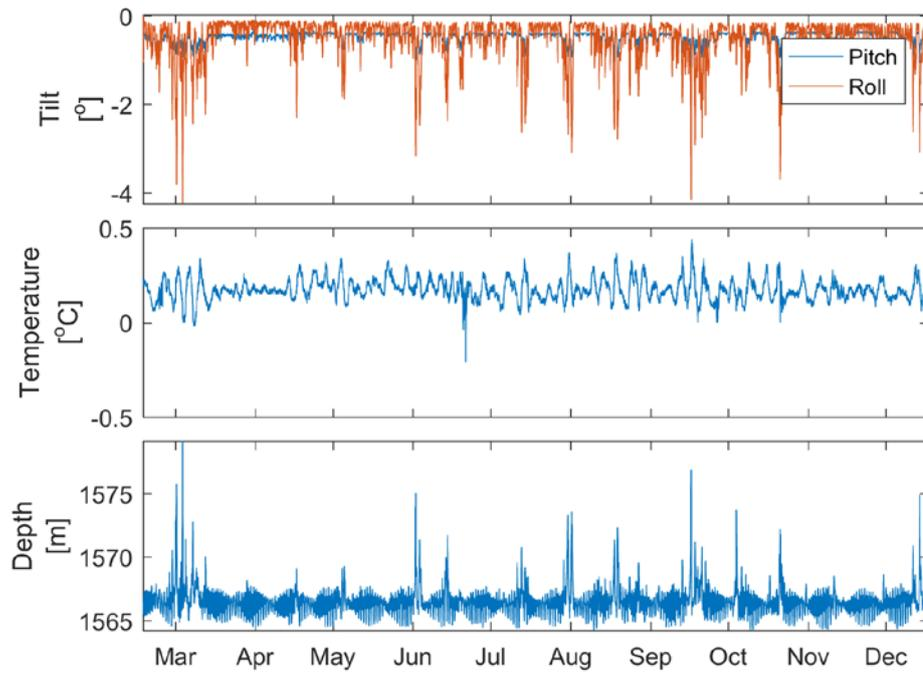
Figure 14. RDI ADCP SN 11434. Time series from tilt, temperature and depth sensors.
