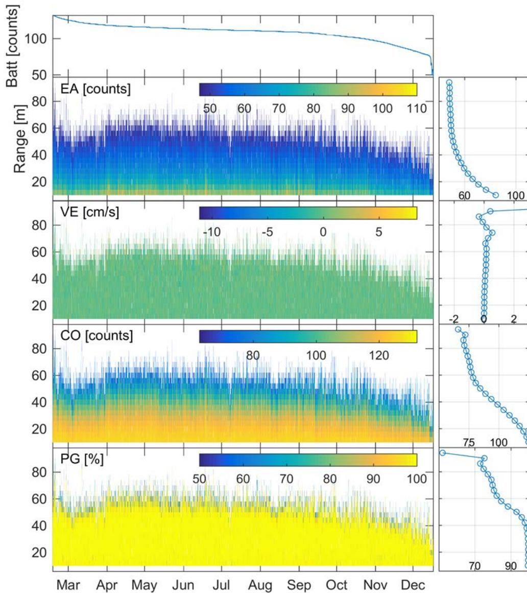
Figure 10. RDI ADCP SN 10149. Time series of battery power in counts followed by vertical range-time maps of echo amplitude, error velocity, coherence (all averaged over 4 beams) and percent good parameter. Rightmost panels show their time average profiles.
