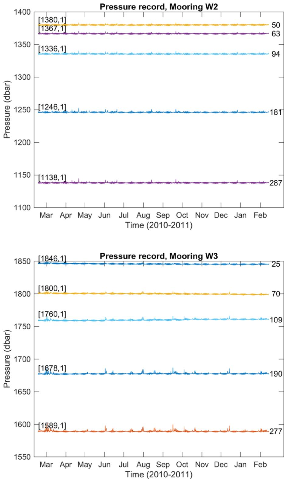
Figure 2. Pressure time series from instruments equipped with pressure sensors, for moorings W2 to W3 as indicated. Time average and one standard deviation values are given in square brackets. The numbers at the end of each record is the height (m.a.b) of the sensor.
