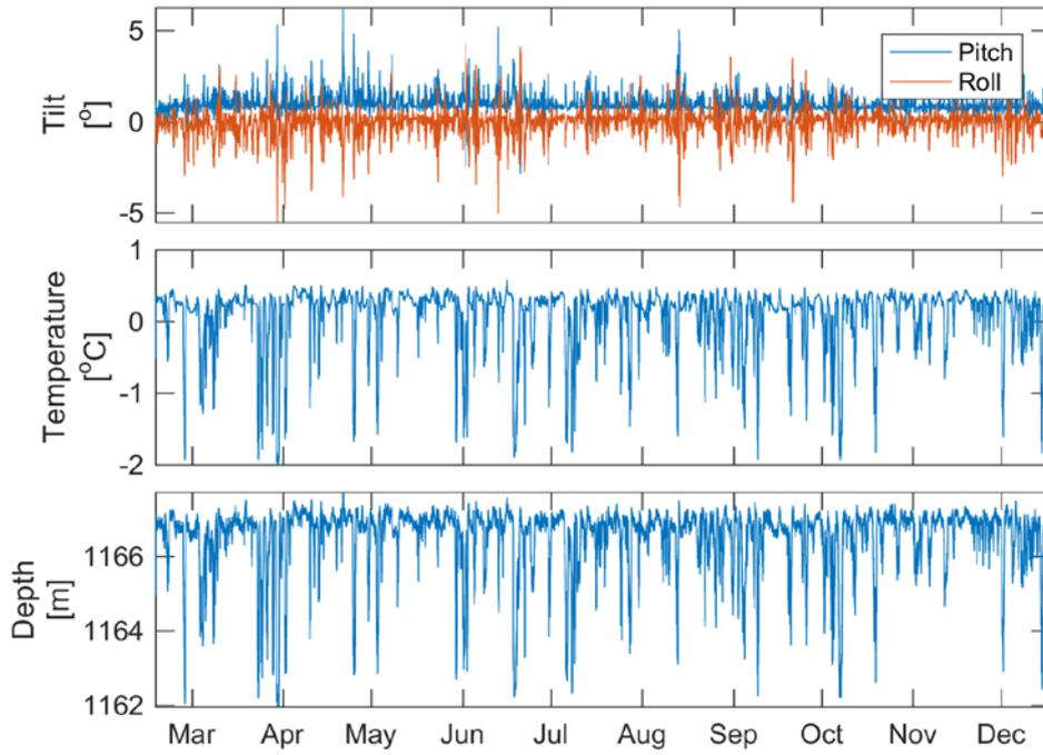
Figure 11. RDI ADCP SN 10149. Time series from tilt, temperature and depth sensors.
