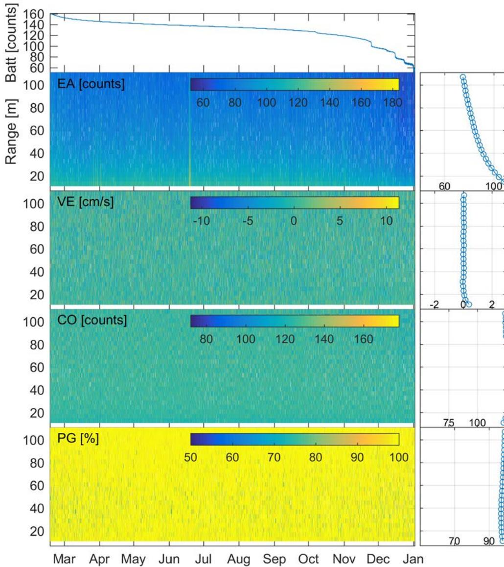
Figure 7. RDI ADCP SN 8645 (Longranger). Time series of battery power in counts followed by vertical range-time maps of echo amplitude, error velocity, coherence (all averaged over 4 beams) and percent good parameter. Rightmost panels show their time average profiles.
