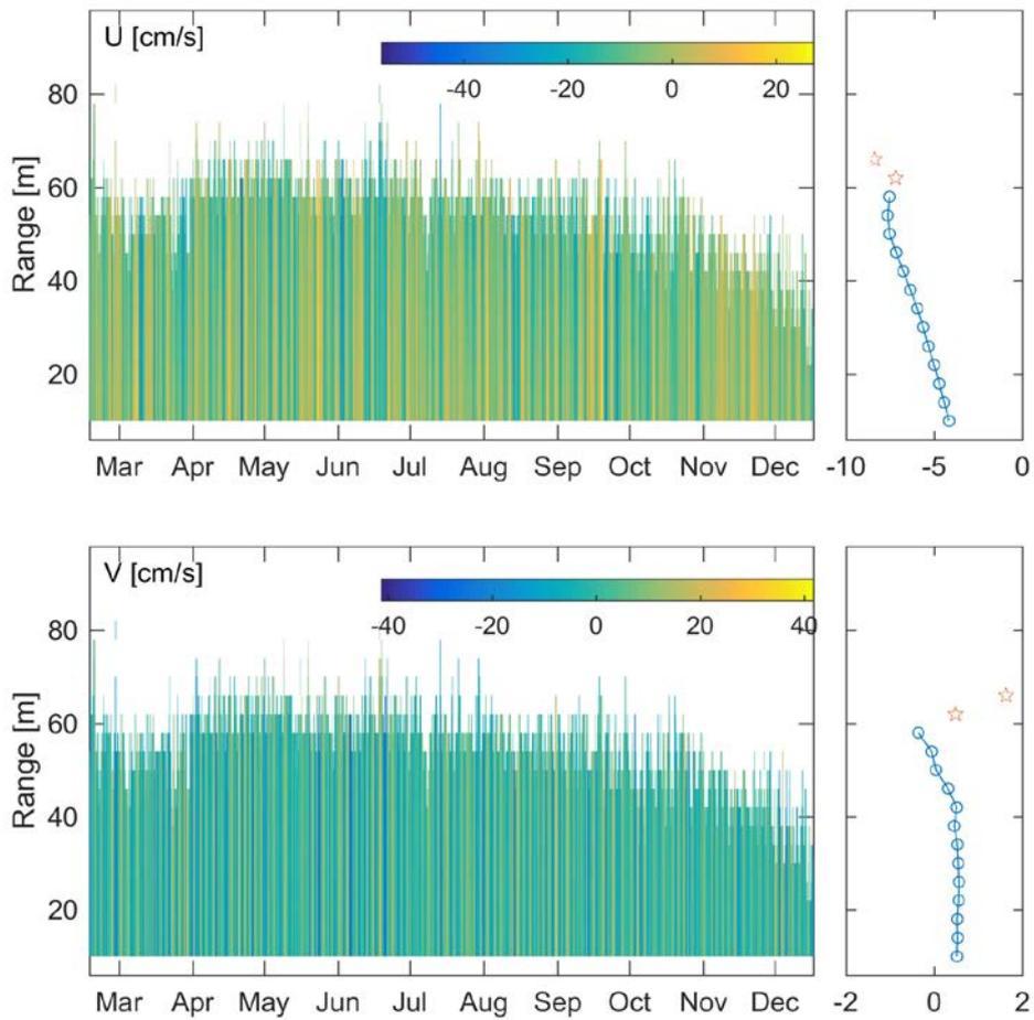
Figure 12. RDI ADCP SN 10149. Vertical range - time maps of east and north velocities and their time average profiles. Pentagram: time coverage between 5-20%.
