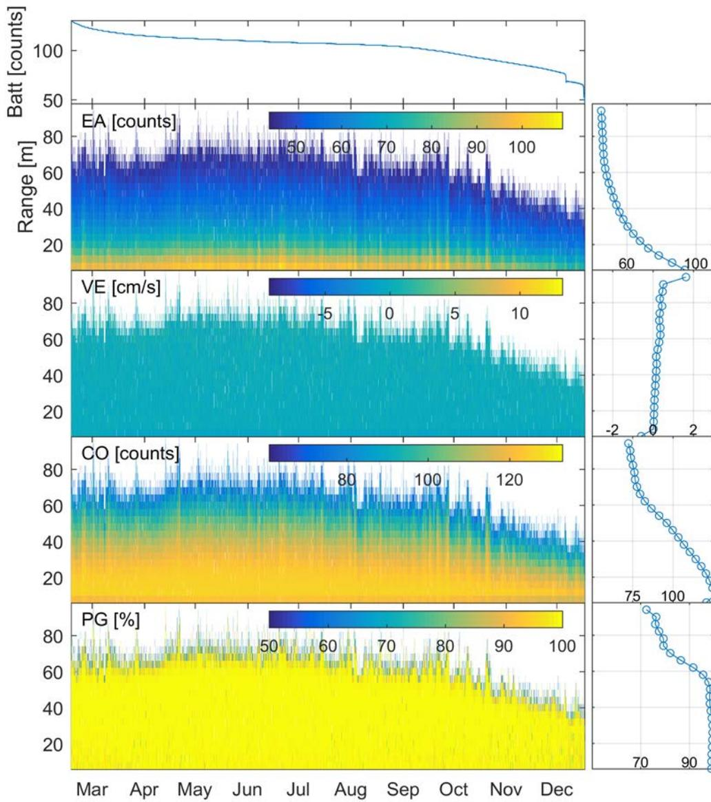
Figure 13. RDI ADCP SN 11434. Time series of battery power in counts followed by vertical range-time maps of echo amplitude, error velocity, coherence (all averaged over 4 beams) and percent good parameter. Rightmost panels show their time average profiles.
