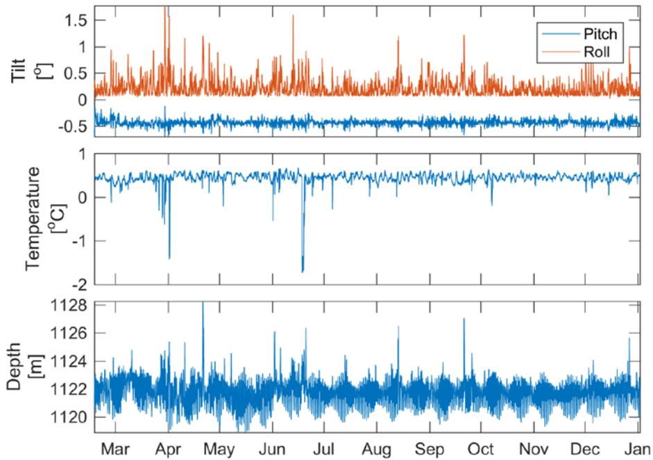
Figure 8. RDI ADCP SN 8645 (Longranger). Time series from tilt, temperature and depth sensors.
