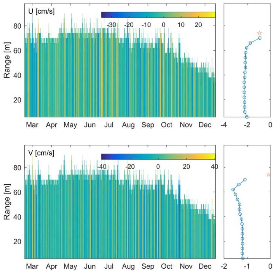
Figure 15. RDI ADCP SN 11434. Vertical range - time maps of east and north velocities and their time average profiles. Pentagram: time coverage between 5-20%.
