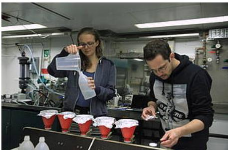
Fig. 2 (23. Jan. 17, 18:22): Sea water samples are filtered on glass fiber filters for further analysis. (Photo: Tom Ehrhardt)
