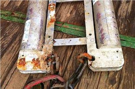
Fig. 6: (27 Jan 17, 15:35): The double release package after its 6-year deployment. (Photo: Olaf Boebel)
