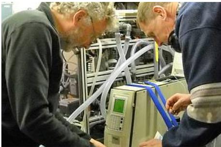
Fig. 1 (22 Dec. 16, 14:20): Calibration of the Systema  $\mu\text{MAC1000}$  Analyzer (provided by M. Gehring, GKSS) for measurements of ammonium in the oceanic surface waters. (Photo: Marion Kreilein)
