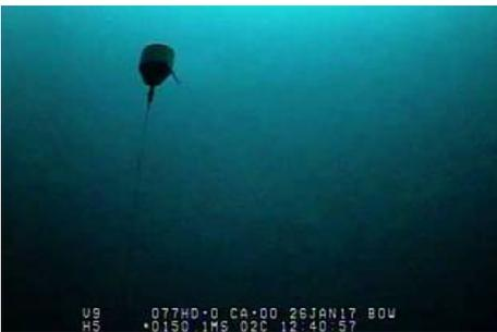
Fig. 4 (26 Jan 17, 12:40): Screenshot of Fiona's video with the mooring's upward looking sonar viewed from about 150m depth - standing out against the blue sea surface. (Photo: Fiona@AWI)
