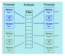
Example of an ensemble integration with two ensemble members. Both models and the filter are parallelized. The ensemble adds one level of parallelization to integrate all members at once.
