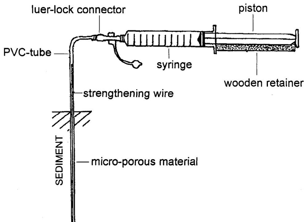
Fig. 4. Schematic of Rhizon sediment moisture sampler
