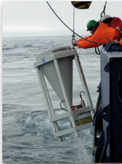
Fig. 9.2: Deployment of a sediment trap to assess particle fluxes to the seafloor
