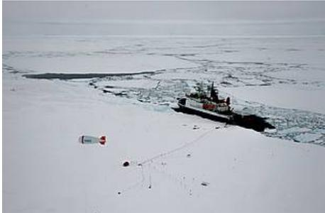
Fig.1.: Polarstern at the ice floe and parts of the ice station, most visible the red tomato and the surrounding meteorology and radiation sites as well as the tethered balloon. (Photo: Stephan Schön - SZ)
