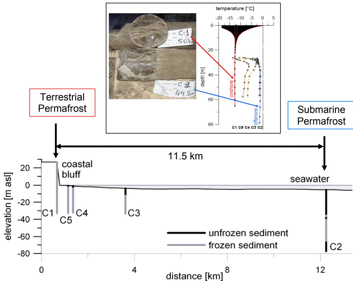
**Figure 4. (above)** Drilling cores and their depth; core C1 is terrestrial permafrost and core C2 is submarine permafrost. The drilling sites are 11.5 km apart; the other cores C3, C4, and C5 were not used in this dissertation (Overdiun et al., 2008, modified); in the photograph similarities in deposits in the permafrost and terrestrial permafrost can be seen (the temperature difference between cores is approximately 10°C (Rachold et al., 2007)
