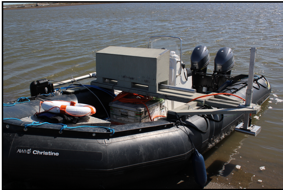
FIGURE 3.3: The Parametric Echosounder Innomar SES-2000 mounted onto the AWI vessel "Christine" that was used to record the profiles in the Herschel Basin in 2013 (Photo by M. Fritz).
