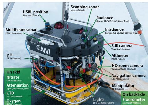
Light transmittance was measured typically under a 100x100 m survey area, covering a wide range of current ice conditions including thin ice, pressure ridges and melt ponds. Ice thickness was derived from the upward looking sonar and the vehicle's depth sensor. Ice relative position was measured with an acoustic ultra short baseline (USBL) positioning system.
