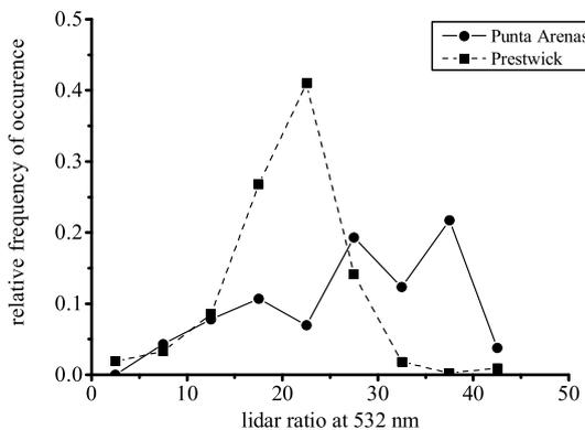
Fig. 3: Relative frequency of occurrence of the lidar ratio of cirrus clouds determined with the lidar at the NH and SH locations.
