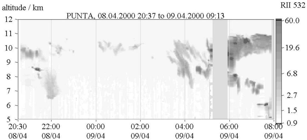
Fig. 1 Lidar measurements of cirrus clouds in Punta Arenas on April 4th 2000. Plotted is the backscatter ratio as a function of time (UT) and altitude. Between 00:00 and 02:00 thin, subvisual cirrus were detected, at an altitude of around 10 km.
