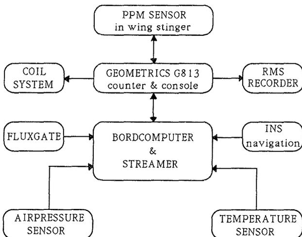
Fig. 2: Data acquisition structogram.
