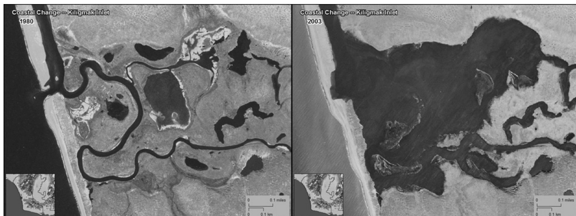
Figure 1. Flooding of Kiligmak Inlet, in Cape Krusenstern National Monument. The infra-red aerial photograph at left shows the creek, inlet, and surrounding tundra as they existed in 1980. The same area in 2003 is shown at right, after a storm moved sand and gravel across the inlet, forming a new lagoon, and flooding the tundra. The new lagoon is about 0.5 km wide.
