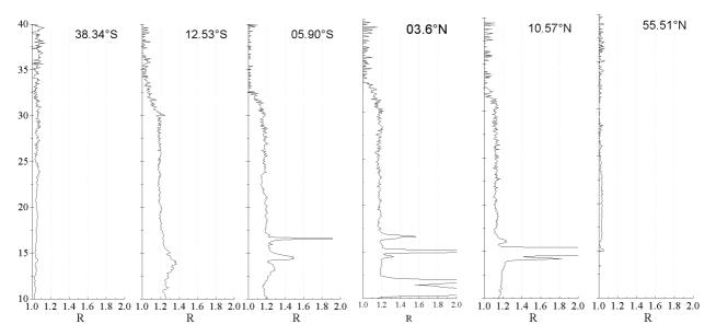
Fig. 4 Backscatter ratio profiles from different latitudes from South to North. While the aerosol load in the midlatitudes is below the detection limit, there is a significant amount of aerosol in the tropical lower stratophere.
