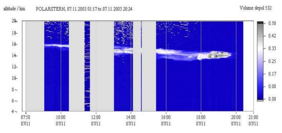
Fig. 2 Volume depolarization at 532 nm measured by the lidar on Nov 7 2003 as a function of time and altitude. A weak but significant signal from is detected from an ultra-thin cirrus. Its optical depth is estimated to  $\tau = 10^{-4}$ . At 18:00 UTC the properties of the cloud change abruptly and it becomes a thick visible cirrus and then disappears.
