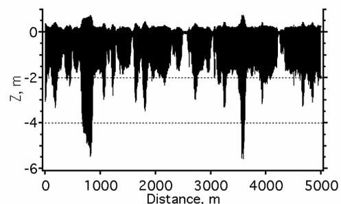
**Figure 6:** Section of a typical ice thickness profile obtained with the EM Bird. For illustration purposes, ice thickness was transformed into freeboard and draft by assuming an ice density of  $880 \text{ kg/m}^3$ . 2.0 m representative for second- and multiyear ice and a small peak at 1.2 m
