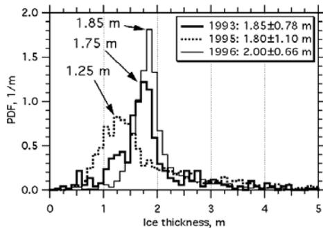
**Figure 2:** Thickness distributions of first-year ice in the Laptev Sea (Haas and Eicken, 2001). The Figure caption shows the mean thickness and standard deviation.
