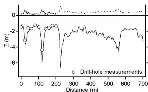
**Figure 1:** Typical ground-based EM thickness profile (Haas and Eicken, 2001). Circles show drill-hole thicknesses obtained for validation of EM estimates.
