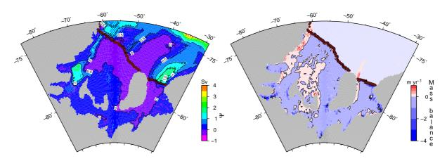
Figure 3: Vertically integrated mass transport stream function (left) and basal melt rate (right) for the control run  $S_{CR}$ .
