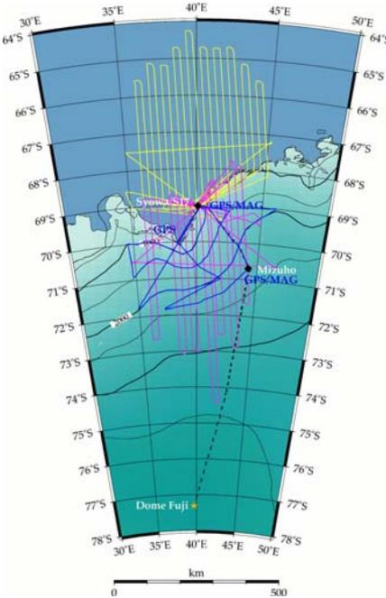
Fig. 3: Survey flights of the ANTSYSO I project: blue lines DISTINCT, yellow and purple lines WEGAS.
