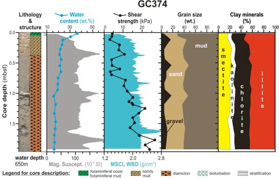
**Figure 2.** Lithology, physical properties (magnetic susceptibility, water content, shear strength, WBD =wet bulk density, measured with the MSCL =multi-sensor core logger), grain-size distribution and clay mineral composition of core GC374 (see Fig. 1 for site location).
