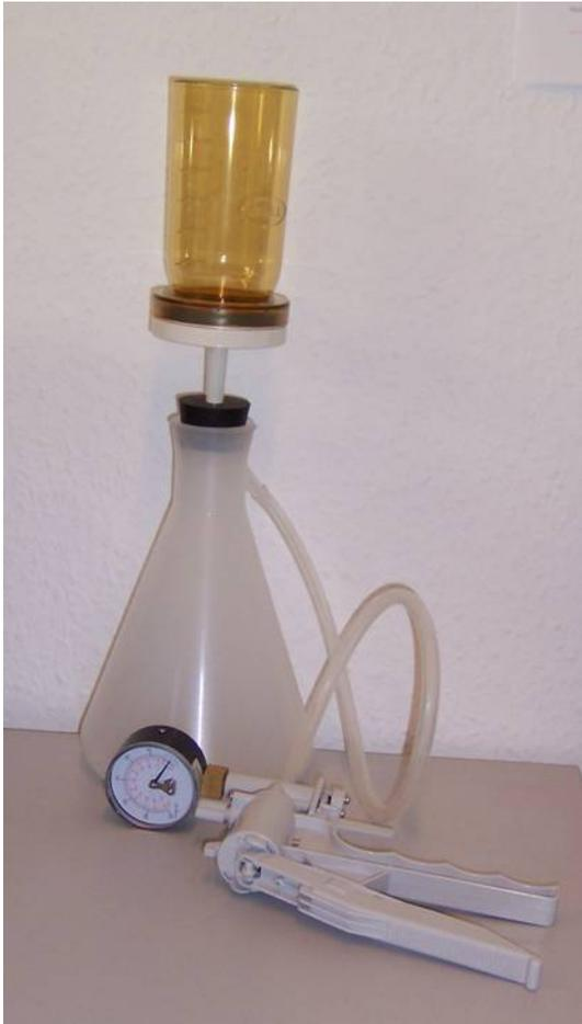
**Figure 2.** Filtration equipment and filtration device
