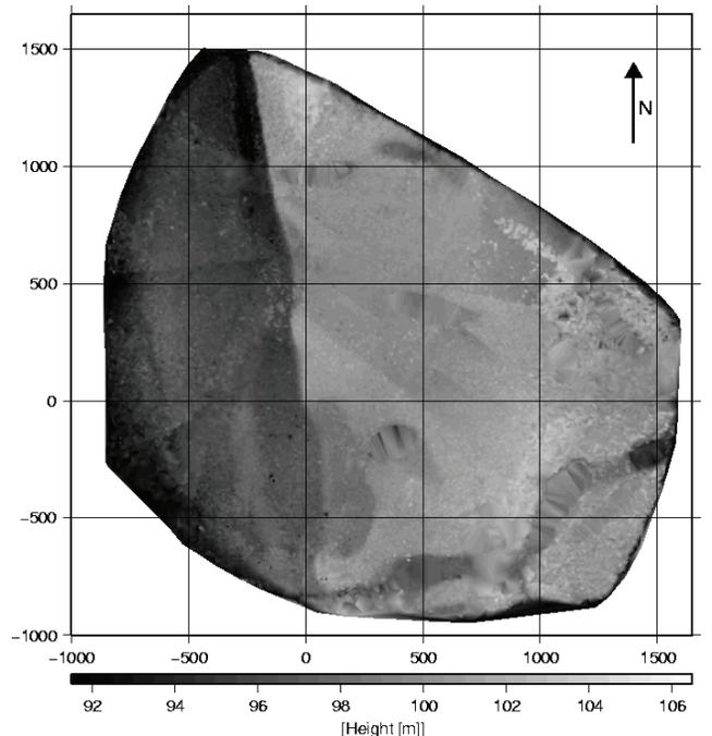
Figure 7. Surface of Samoylov Island:  $x$ - and  $y$ -coordinates are in a local coordinate system (scale in m). The heights of the points of the DEM are relative heights with respect to the origin of the local coordinate system (0.0) with a height of 100 m.
