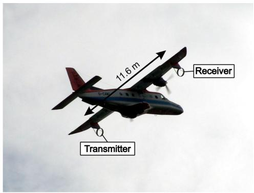
Figure 1. AWI Dornier 228 with the fixed wing sea ice thickness system
