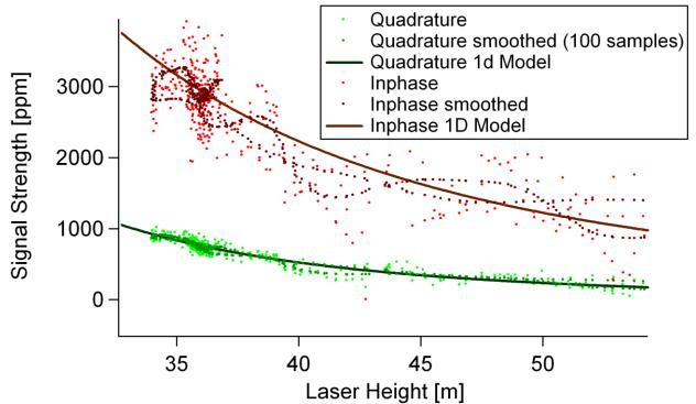
Figure 2. Modelled and measured Inphase and Quadrature signal in ppm plotted against altitude over open water in m.
