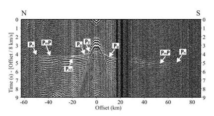
**Figure 4.** Airgun shots recorded by OBS 105. Phases  $P_g$ ,  $P_n$ , and  $P_mP$  are as in Figure 3.  $P_2$  corresponds to P waves refracted in the upper crust low-velocity sediments, and  $P_{c2}$  P waves are reflected inside the crust (notation from *Parsiegla et al.* [2007]). Reduced traveltimes are shown with a reduction velocity of 8 km/s.
