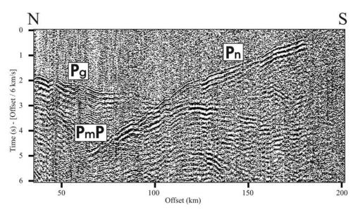
**Figure 3.** Example of the data from airgun shots picked up by land receiver 46. Direct P waves from the crust  $(P_g)$ , from the mantle  $(P_n)$ , and Moho reflections  $(P_mP)$  are clearly visible. Reduced traveltimes are shown with a reduction velocity of 6 km/s.
