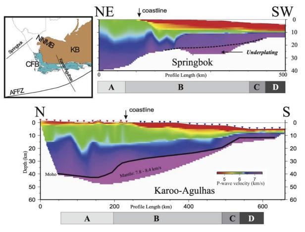
**Figure 11.** P-wave velocity model comparison between (top) the Springbok profile on the western coast of South Africa [after *Hirsch et al.* 2008] and (bottom) this study. On the basis of Moho geometry, four segments of the crust can be distinguished in both profiles: (A) thick continental, (B) stretched gradually thinning, (C) steeply thinning, and (D) thin oceanic crust.
