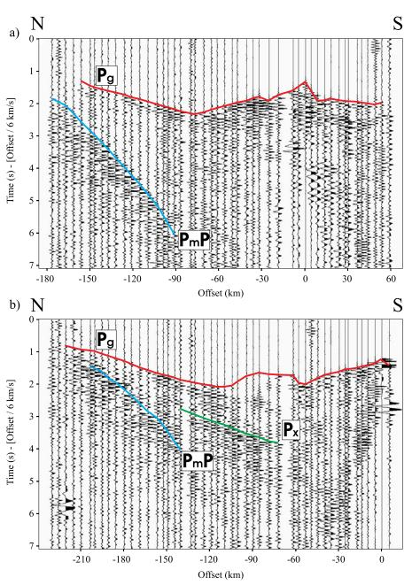
**Figure 2.** Examples of data recorded by land receivers from land shots. (top) Shot X10. The refracted P waves ( $P_g$ ) are marked in red, and Moho reflections ( $P_mP$ ) are in blue. (bottom) Shot X13. Phases reflected off the "floating" crustal reflector ( $P_x$ ) are marked in green. Reduced traveltimes are shown with a reduction velocity of 6 km/s.
