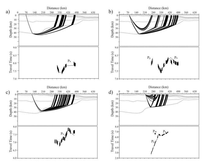
**Figure 8.** Airgun shots recorded by 4 land receivers: (a) receiver 12; (b) 17; (c) 24; (d) 44. (top) The raypaths; (bottom) the observed traveltime (steeples corresponding to uncertainty bars) and the traveltime expected from the model for the given source-receiver distance (solid line).
