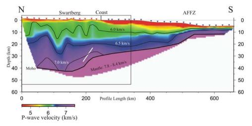
**Figure 7.** P-wave velocity model for the entire profile. To help the location with Figure 1, land shots (red triangles) and OBSs (blue triangles) have been indicated. Velocity contours corresponding to 6.0, 6.5, and 7.0 km/s have been drawn. The thick white line marks the "floating" reflector. The black rectangle indicates the northern 340 km that is shown in Figures 5 and 6.
