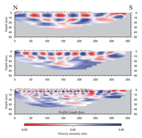
**Figure 6.** Resolution tests for the model in Figure 5. Original checkerboard sizes are (top)  $40 \times 10$  km, (middle)  $25 \times 10$  km, and (bottom)  $12 \times 5$  km; velocity perturbation of 5% is used in each case.
