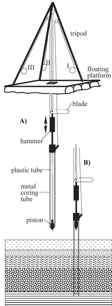
Fig. 4: Sketch of the coring gear and process.
