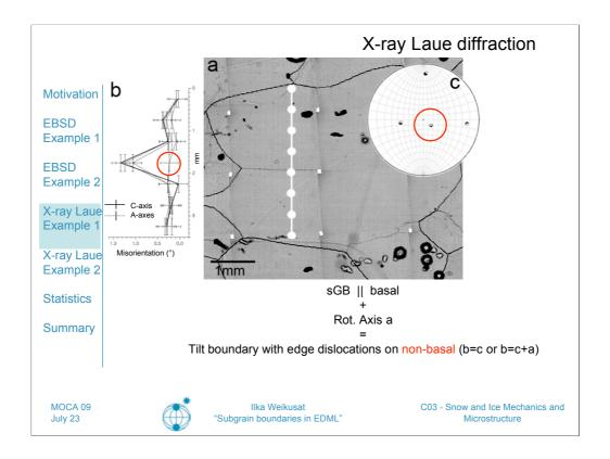
Same result found with X-ray Laue diffraction (oldest crystallographic method can be applied to polycrystalline ice, because of large grain sizes compared to other materials)
