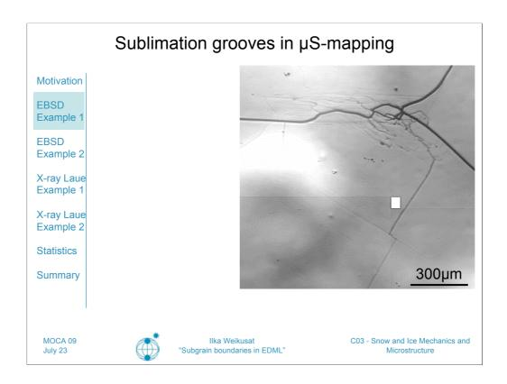
grooving under sublimation due to thermal etching
