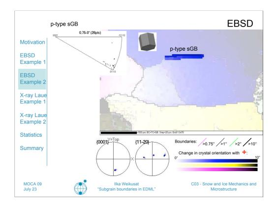
Texture component map Focus on blue grain Overall crystal orientation
