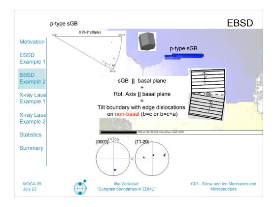
RotAxis AND sGB plane || to basal plane cannot be explained with basal dislocations
