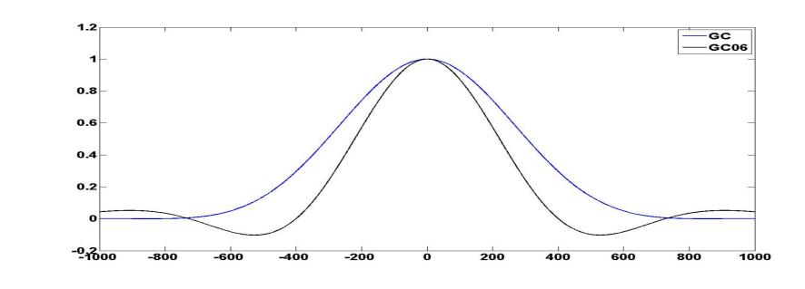
Correlation functions used for weighting of observations: 5th order polynomial weighting (blue line), and weighting using correlation model from [1] as shown with black line.
