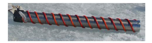
Figure 3.4: 9 cm diameter corer (Photo: Camille Fresser)
