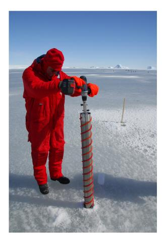
Figure 3.5: Drilling a sackhole with an ice corer (Photo: Camille Fresser)
