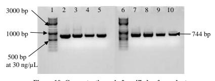
**Figure 10: Concentration gel of purified** *egfp* **product, showing roughly 200 ng/µL PCR product.** Lane 1+6: Ladder; Lane 2-5: sample 1-4; Lane 7-10: sample 5-8.
