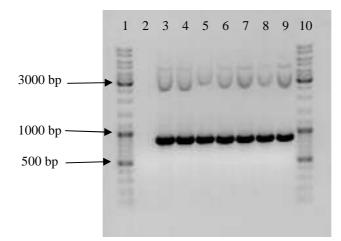
**Figure 9: Temperature gradient PCR for the amplification of the resistance gene** *neo* **from 200 ng of the commercially available plasmid pSELECT (InvivoGen, Germany).** Lane 1+10: Ladder; Lane 2: neg. control; Lane 3: 51.2°C; Lane 4: 51.7°C; Lane 5: 52.6°C; Lane 6: 53.7°C; Lane 7: 55.0°C; Lane 8: 56.4°C; Lane 9: 57.8°C.
