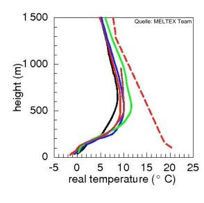
Vertical temperature profiles over land (----) and over sea ice; heat flux towards the ice surface
