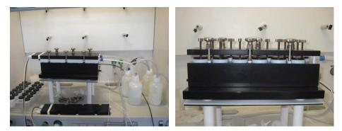
**Figure S 1:** *left: Experimental setup for preconcentration of liquid samples before the addition of acids and after acid digestion. Right: Experimental setup for the acid digestion of Antarctic ice core samples.*
