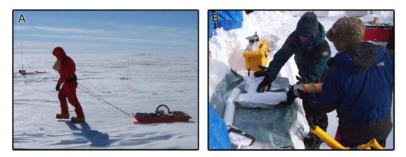
Figure 1.3.: Ground-based activities during CryoVex 2004. (A) The man-pulled sledge hosting GPR and GPS-systems. (B) Retrival of a shallow firm-core for physical properties measurements.
