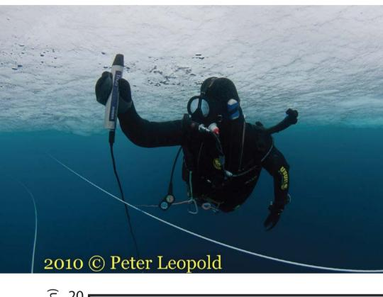
Divers measured the spectral flux transmitted to the underside of first-year pack ice floes along well-defined profiles covering heterogeneous regions (melt ponds, ridges and other features). Incident flux at the surface was measured at the same time. After the dive, ice and snow properties were measured along the profile.
