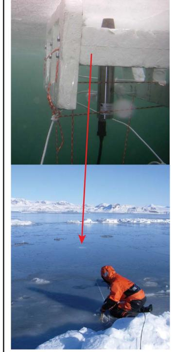
Transmitted light was measured using an under-ice floating sled pulled between holes made in the ice, allowing undisturbed measurements under thin (4-40 cm) level ice. A folding arm was used for thicker first-year ice. Surface irradiance was measured simultaneously with a second sensor.
