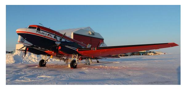
**Figure 2.1.:** Polar-5 in Barrow during SIZONet 2011. The EM-Bird can be seen below the aircraft body.
