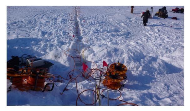
**Figure 3.13.:** Photo of ERT setup. Shown are the electrodes between y = -25m and y = 0m
