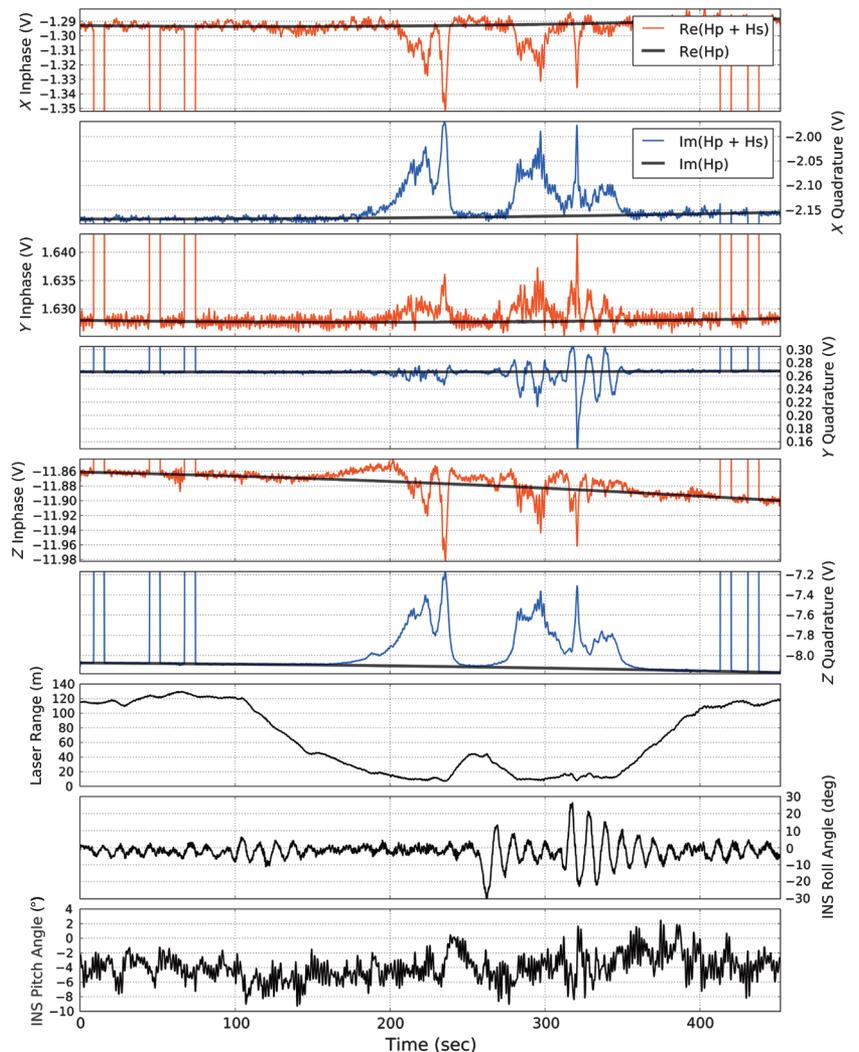
Figure 7. Example of raw data from all three receiver components ( $x, y, z$ ) of the in-phase (red) and quadrature (blue) channels at 4.1 kHz in multifrequency mode (top six panels). The received voltages are provided as secondary and primary field ( $H_p + H_s$ ) and the residual primary field ( $H_p$ ) for about eight minutes. The lower three panels show the altitude measured by the single-beam laser altimeter and the roll and pitch angles sensed by the INS.
