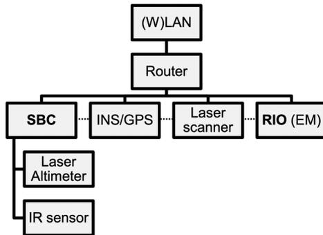
Figure 5. Data acquisition schematics. Black lines indicate data connection (Ethernet, RS232, or USB) between sensors and DAQ units (SBC and RIO). The stippled line indicates the direct PPS connection between GPS and laser scanner, SBC, and RIO for accurate time stamping. Streaming raw data from all five sensors is logged by the SBC and resampled to 10 Hz real-time data sent to the operator computer via WLAN.
