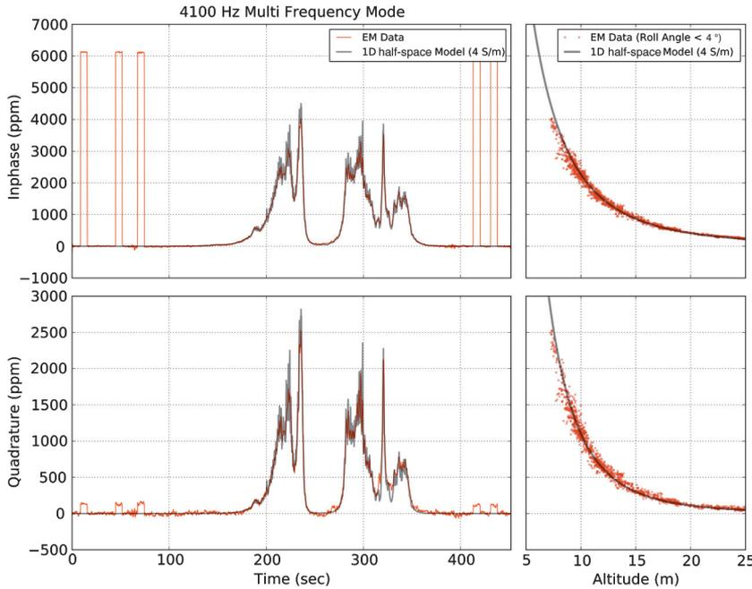
Figure 8. Calibrated and modeled EM response over water ( $z$ -component only) given by in-phase (red) and quadrature (blue) channels at 4.1 kHz in multifrequency mode. The panels on the left side show the comparison of measured and modeled data along the profile; on the right side, the comparison is given as a function of instrument height above the water.
