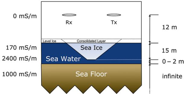
Figure 1. Cross section through 2D pressure ridge geometry used for the EM modeling study. The geometry of the ridge is typical of observed natural ridges (max width =  $4 \times$  thickness, min width = thickness/2). The HCP system height is a constant 12 m above the water table.
