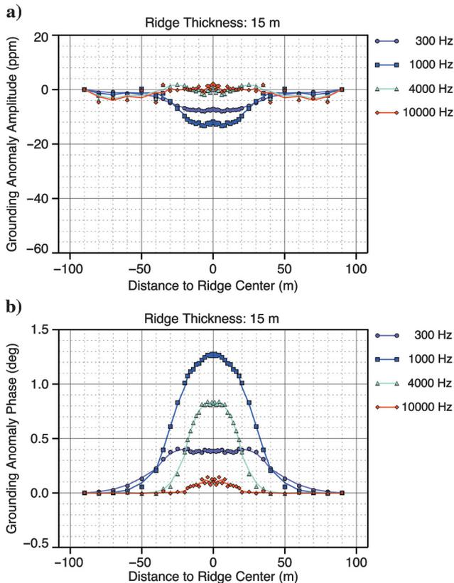
Figure 2. Ridge grounding anomaly (i.e., the difference in EM response for a grounded ridge compared to a floating ridge with 2 m water below the keel) for 15 m ridge thickness at signal frequencies 300 Hz to 10 kHz. The upper and lower panels show the normalized secondary field expressed as (a) amplitude and (b) phase component, respectively.
