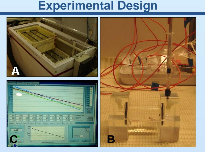
A) Maintenance of krill during starvation experiment (n=48) B) Krill in respiration chamber with oxygen sensor C) Respiration measured over time displayed
