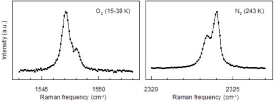
Fig.1 Raman spectra of a clathrate hydrate in Dome Fuji Antarctic ice from 1570 m.
