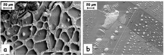
(a) Slowly cooled samples down to -30°C (cooling rate 1.5 K/min, (b) Rapidly cooled samples in liquid nitrogen relative humidity 5% in the glove box).
