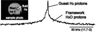
Fig. H2-filled ice II powder NMR spectrum at 2.1 GPa and room T [Fig]
