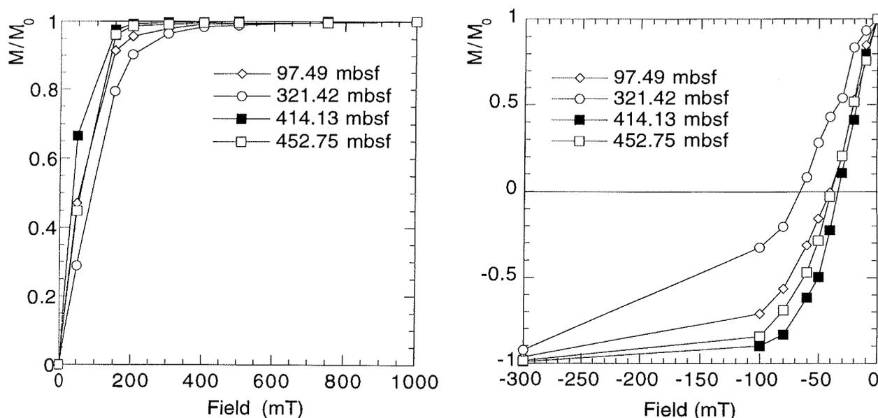
Fig. 8 - Plot of isothermal remanent magnetization (IRM) acquisition and DC demagnetization of representative samples from CRP-2/2A. Some samples have low coercivity ( $B_{cr}$  of about 40 mT) and saturate rapidly (below 300 mT) which indicates the dominance of low coercivity magnetic minerals. Other samples have high coercivity ( $B_{cr}$  of about 65 mT) and saturate above 300 mT, which indicates the presence of significant amounts of high coercivity magnetic minerals.
