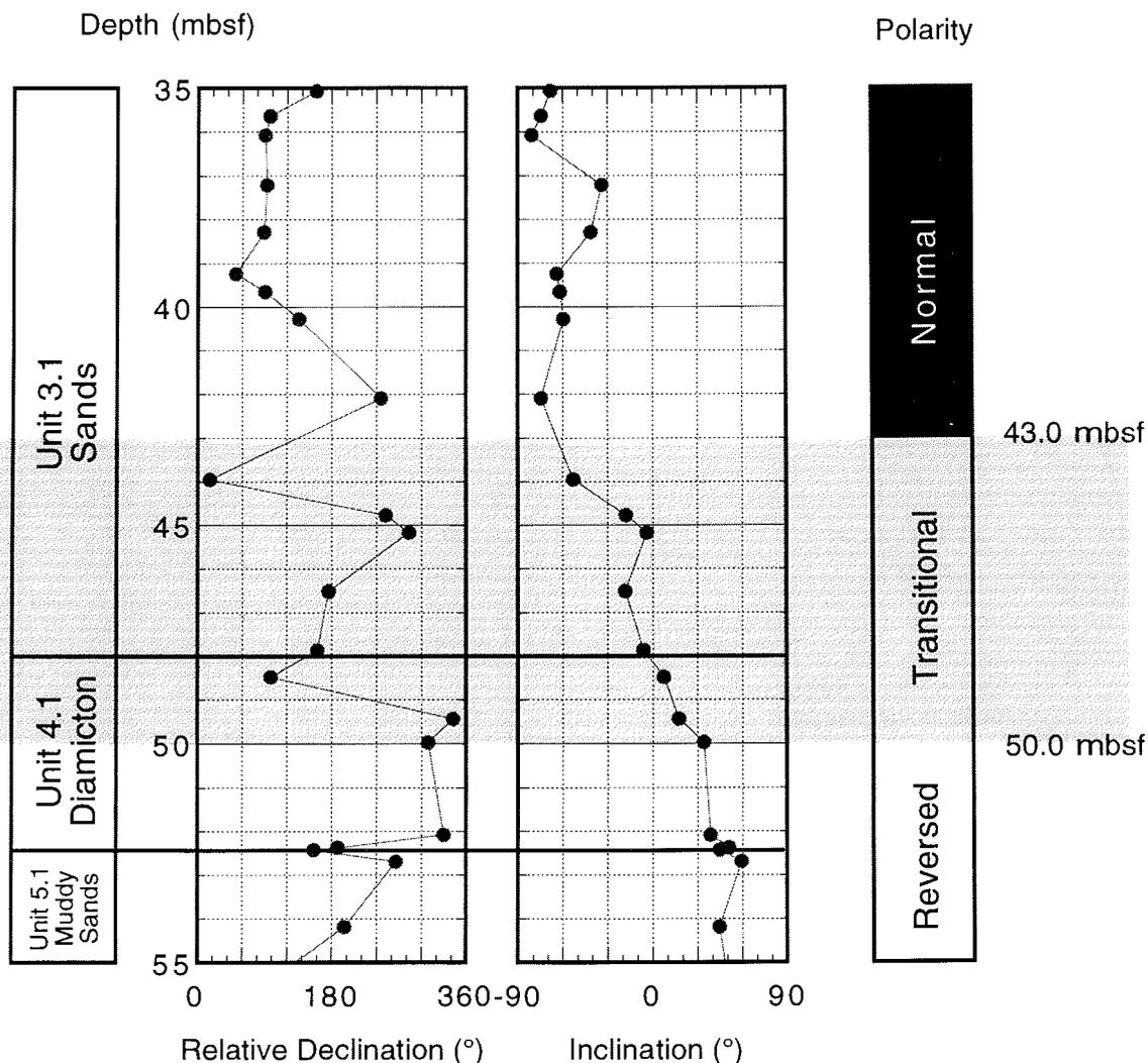
Fig. 7 - Variations in palaeomagnetic declination (arbitrary) and inclination (identified from principal component analysis of multiple demagnetization steps) through the inferred geomagnetic polarity transition (shaded) between magnetozones R2 and N2. The drillcore is not oriented with respect to north. The transition crosses the contact between lithostratigraphic units 4.1 and 3.1 and provides an estimate of accumulation rates and of rates of glacial processes (see discussion in text).
