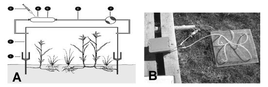
**Figure 7-3**: Scheme of the methane flux measurement set with the closed chamber method (A) and a connected sampling set (B).
