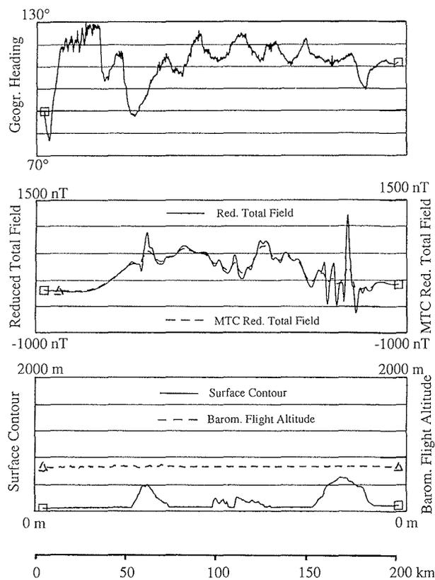
Fig. 3: Section of an aeromagnetic profile over McMurdo Sound, Brown Peninsula, Black and White Islands (for locations see Fig. 1). Aircraft heading (upper part), reduced total magnetic field (middle), and barometric altitude and surface contour (bottom).
