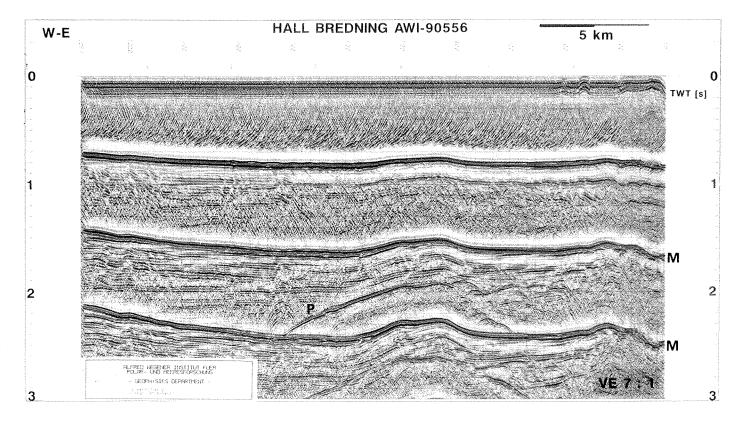
Fig. 4: Line AWI-90556 from southwestern Hall Bredning. Here, some deeper structures can be observed in the Mesozoic sequence (between CDP 700 and 100). Those structures may indicate tectonic movements which are restricted to the southwestern part of Hall Bredning and may thus correlate with the western boundary of the Jameson Land Basin. P = primary reflection, M = ocean bottom multiple.
