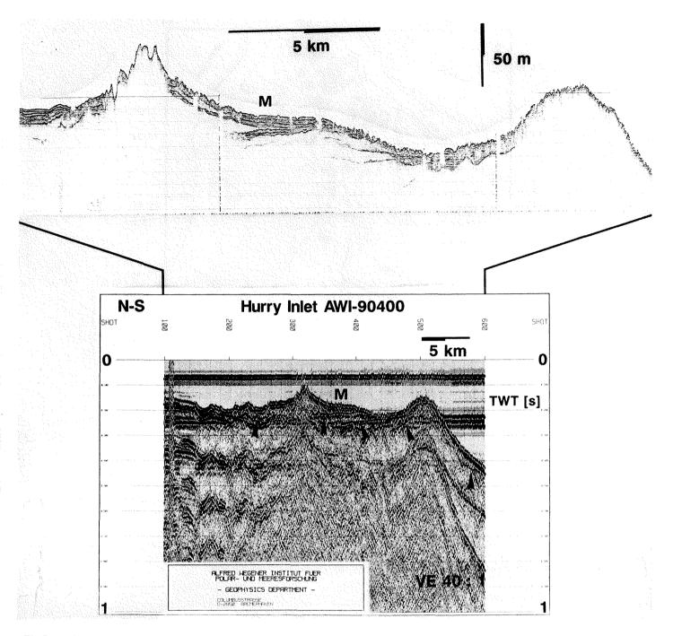
Fig. 7: Moraine structure (M) on line AWI-90400 in the Hurry Inlet. Parasound recording on top of seismic data. The base of the moraine can be clearly identified (Parasound and two left arrows in seismic record). The form of the structure suggests ice movements as well from the north as from the south.
