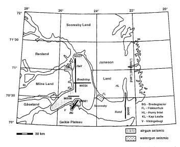
**Fig. 1:** Map of seismic investigated area in Scoresby Sund. Shaded area = airgun seismics, hatched area = watergun seismics. The thick lines show the locations of the profiles referred to in the text. During the whole experiment Parasound data were recorded.
