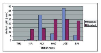
**Fig. 7:** Observed and modelled land uplift for 1995-2001 for the roughly South to North transect of "good" GPS stations along the Nares Strait, relative to Thule.
