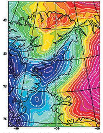
Fig. 8: Geoid heights (meter) in the Nares Strait region from the ArcGP geoid model. Crosses show location of GPS sea-level points.
