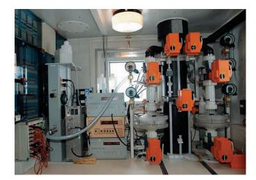
**Fig. 2:** A view inside the air chemistry observatory: Aerosol sampling on filters (right hand), integrating nephelometer and condensation particle counters (left hand).
