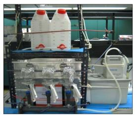
Fig. 5.3: Filtration ramp for CTD water (left) and inline filter holder system (right) on board Polarstern during ARK-XXIII/1
