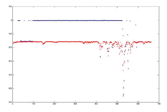
Fig. 3.3: First and last pressure of each CTD-logger record interval (duration 30 min every 12 h). Pressure is in dbar against CTD-logger record number
