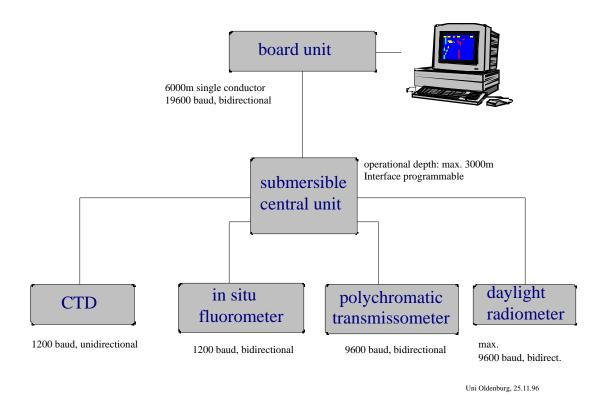
Fig. 7: Coupling of the optical sensors
