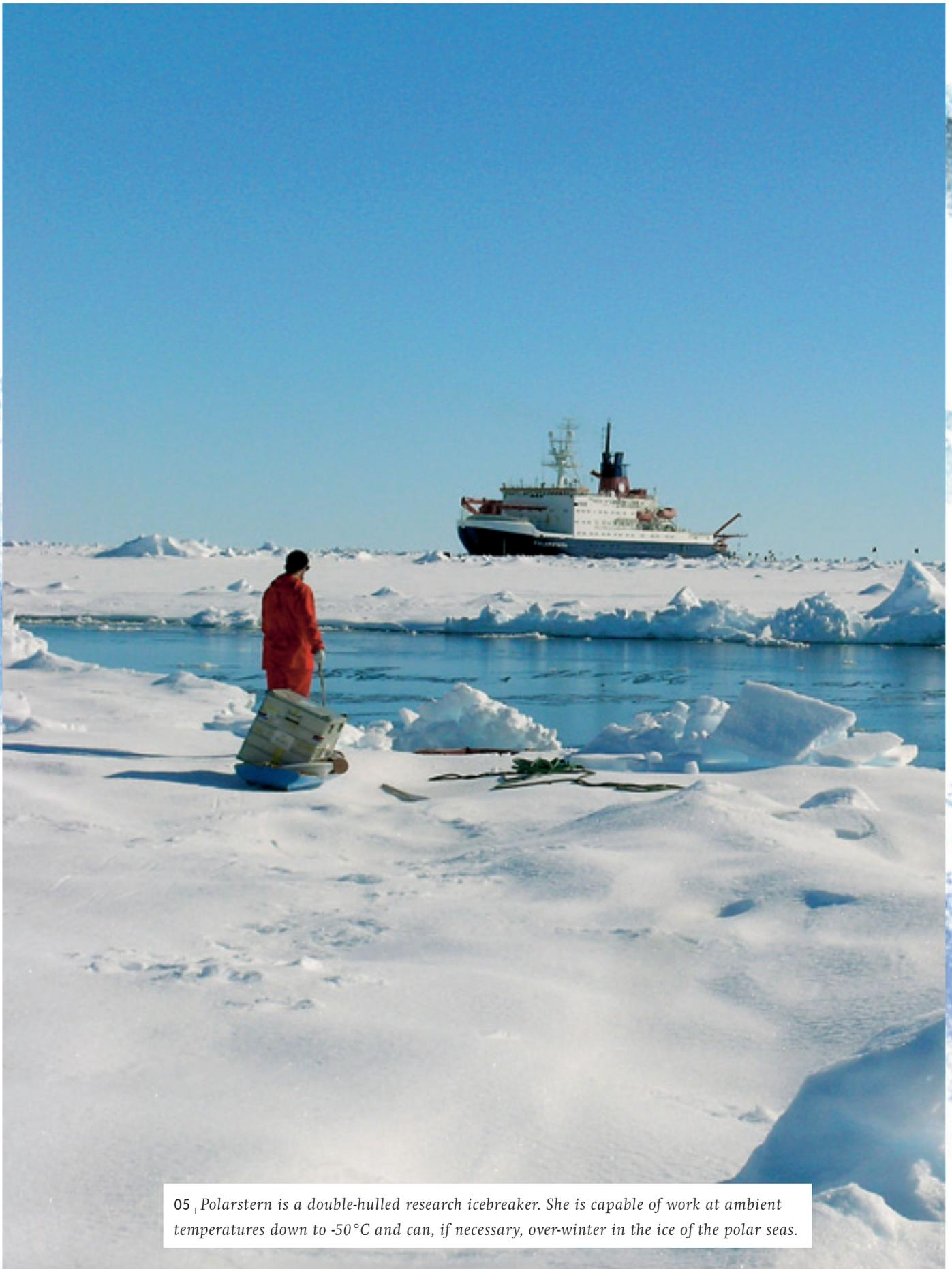
05 | *Polarstern is a double-hulled research icebreaker. She is capable of work at ambient temperatures down to  $-50^{\circ}\text{C}$  and can, if necessary, over-winter in the ice of the polar seas.*
