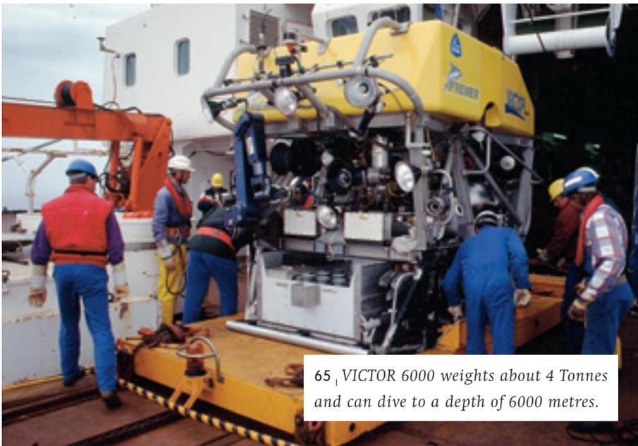
65 | VICTOR 6000 weighs about 4 Tonnes and can dive to a depth of 6000 metres.
