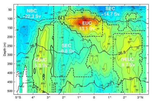
Figure 6 Zonal velocity component from the vessel mounted 75kHz Ocean Surveyor. The bold dark lies are isopynals, separating the Subtropical salinity maximum water from the central water masses. Below the sigth= 27.1, the Antarctic Intermediate Water (AAIW) is located. Positive: eastward flow, negative: westward flow.
