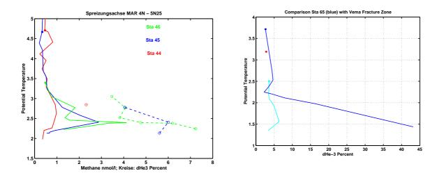
Figure 9 helium and methane profiles from the MAR: left  $4^{\circ}N - 5.5^{\circ}N$ , bold lines: methane, stippled lines: helium. Right side: helium in the Vema fracture zone (light blue line), the high values at the bottom of more than 40% are from the spreading axis just north of the Vfz (dark blue line). Note the different scale of the xaxis.
